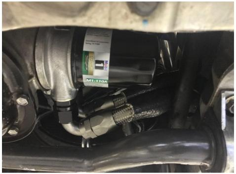
12. With one side of the lines hooked up, take the other side of the lines and wrap them over the front impact bar and in between the radiator/condenser and the vertical center brace for the front core support, where the top of the cooler core will mount.
