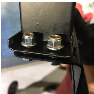
14. Attach the upper bracket to the cooler cure with the two supplied 10mm bolts and lock nuts. At the same time take the small section of rubber edging and cut a slit down the middle and slot it into the small gap on the upper bracket.
