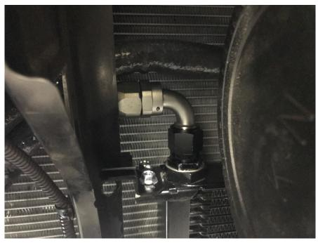
20. Now with the cooler in position, screw the two 10mm bottom mounting bolts into the barrel nuts installed in step #17.
