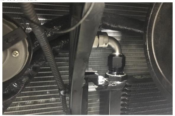
13. Attach the lower mounting bracket to the cooler core with the four supplied 10mm bolts and lock nuts **make sure** to insert the bolts from the bottom to avoid clearance issues. Use the 4 rubber washers in between the bracket and the cooler core to insulate the assembly.
