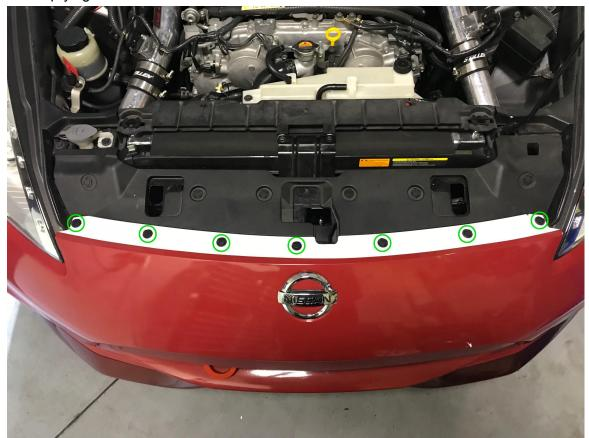
3. Lift the car and remove the ten 10mm bolts along the bottom of the bumper cover (yellow circles), the eight 10mm bolts holding on the splash shield (red), as well as the three plastic pop clips also holding the splash shield in place (green).
