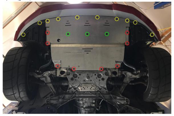
4. Carefully remove the bumper cover. There are clips located next to the where the mounting bolt was as well as below the headlight. A small tug on each side should pop the bumper loose.
